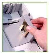
The paper trays can hold a maximum of 520 sheets of 20 lb (80 g/m<sup>2</sup>) bond paper. **3.** If necessary, open the back of the paper tray to allow for paper sizes such as Legal, Oficio and Folio. Adjust the rear guide.
