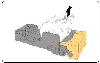
4. Insert a new staple cartridge into the staple case.
