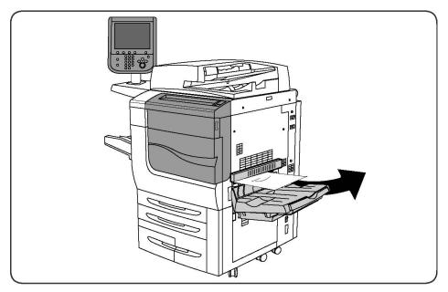
2. If paper is torn, check for any torn pieces of paper inside the machine.
