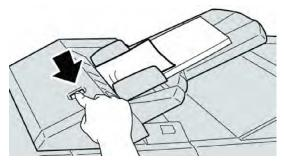
2. Open cover **1e** and then remove the jammed paper and all paper loaded in the tray.
