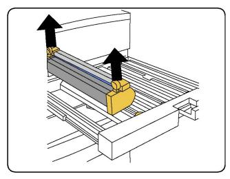
9. Place the new drum cartridge in the machine following the guides with the side marked front facing the front.
