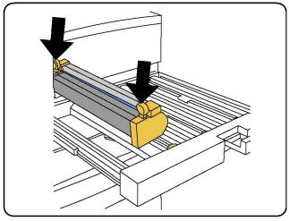
10. Press both ends of the drum cartridge to place it in a horizontal position.
