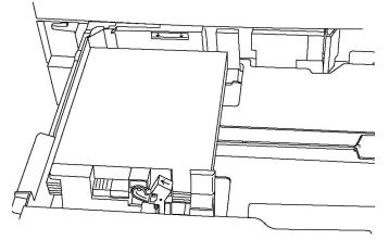
5. Adjust the guides so they touch the edges of the stack.
