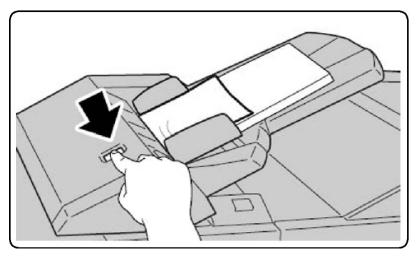
2. Open the cover and remove the jammed paper.
