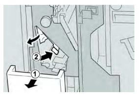
If paper is torn, check inside the machine and remove it.
