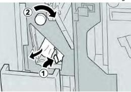
5. Return the opened lever (**2f**) or (**2e**) to its original position, and close the output tray (**2d**).
