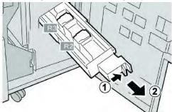
4. Hold the tabs of the staple cartridge unit by the tabs and lift to remove it.
