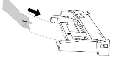
4. Adjust the width guides until they just touch the edges of the stack.
