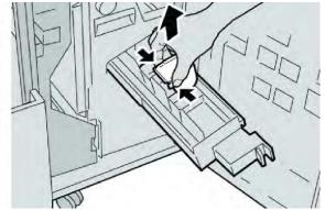
5. While holding the tabs of a new staple cartridge, push it into the unit.
