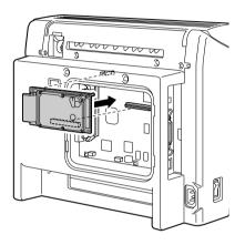
8 Reinstall the panel and tighten the screw.
