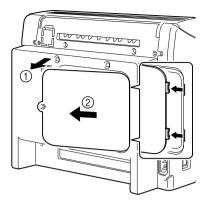
4 While holding the tab on the hard drive mounting pin slid to the left, remove the hard drive.
