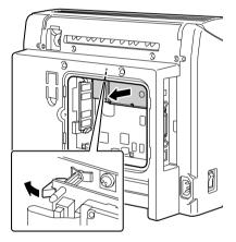
5 Remove the backup battery from the back of the hard drive.
