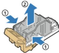
5. Insert the front side of the new staple refill into the staple cartridge (1), then push the rear side into the cartridge (2).
