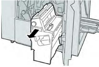
4. Turn the knob **4a** to remove the jammed paper from the left side of unit **4**.
