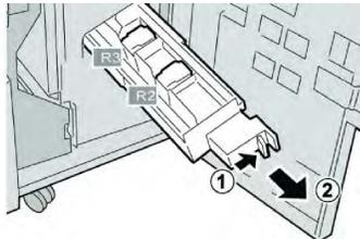
4. Hold the tabs of the staple cartridge unit and lift to remove it.
