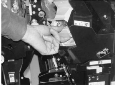
4. Check the inside of the finisher for any remaining staples, and if necessary, remove them.
