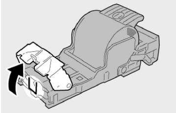
5. Move the lever on the rear of the staple cartridge unit in the downward direction.
