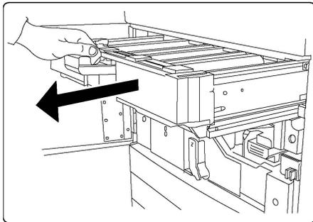
6. Grasp both of the amber-gold colored casings on the old Charge Corotron and push towards the back of the machine. You will hear a clicking noise indicating that it is being released.
