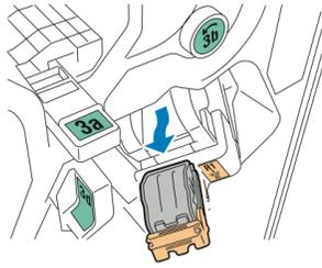
4. Pinch both sides of the staple refill (1) and remove it from the cartridge (2).
