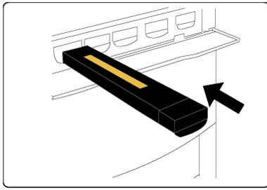
8. Close the Front Door. If the door will not close completely, make sure the cartridge is in the lock position and the toner cartridge is installed into the appropriate toner location.
