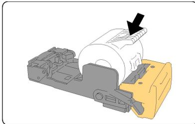
6. Reinstall the cartridge unit to its original position in the finisher.
