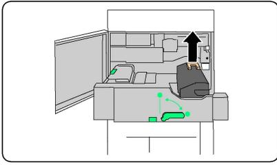
5. Dispose the Fuser as normal office waste or recycle the fuser.
