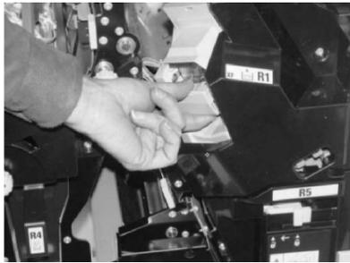
4. Hold the positions as indicated by the arrow and remove the staple cartridge from the unit.
