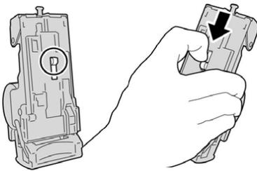
6. While holding the lever down, turn over the unit and remove the staple cartridge from the unit.
