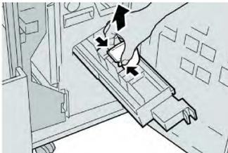
5. While holding the tabs of a new staple cartridge, push it into the unit.
