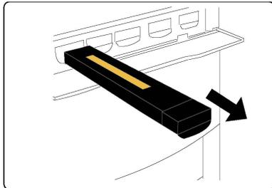
3. Remove the toner cartridge by holding the handle on the top of the cartridge while gently pulling it straight out. Be careful to not get toner on clothing.
