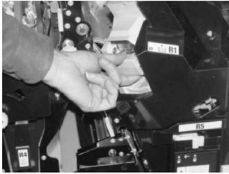
4. If necessary, raise the staple cartridge unit as shown and remove the jammed staple.
