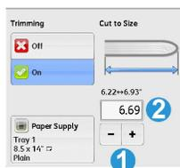
1. Select the buttons to decrease or increase the trimmer setting. Adjustments are made in 0.1 mm/0.0039 inch increments.
