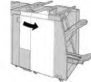
3. Pull out the folder output tray (2d), swing lever 2e/2f to the right, and remove the jammed paper.
