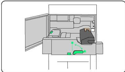
4. Grab and lift the Amber-Gold colored handle only, lift and pull up and out of the Transfer Module.
