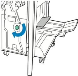
3. To remove the paper, pull it in the direction shown.
