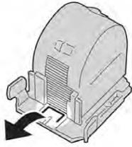
6. While holding the tabs of a new staple cartridge, push it into the unit.
