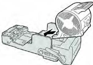
9. Reinstall the cartridge unit to its original position in the finisher.
