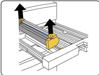
9. Place the new drum cartridge in the machine following the guides with the side marked front facing the front.
