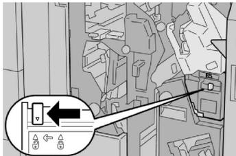
4. Hold **R5** as shown in the figure and remove the staple waste container from the machine.
