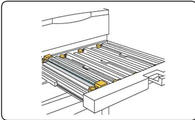
8. Remove the old drum cartridge by holding the finger rings provided at the both ends of the drum cartridge and gently lifting up.
