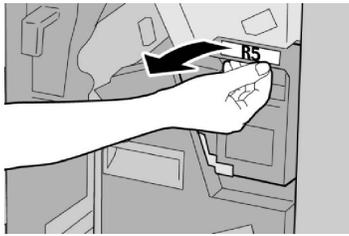
5. Place the used staple waste container into a supplied plastic bag.
