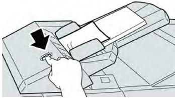
2. Open cover **1e** and then remove the jammed paper and all paper loaded in the tray.
