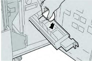
7. Push the staple cartridge unit to its original position in the machine.
