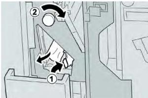
5. Return the opened lever ( 2f) or ( 2e) to its original position, and close the output tray ( 2d).
