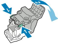
6. To remove the staple refill, press the rear of the refill container as shown.
