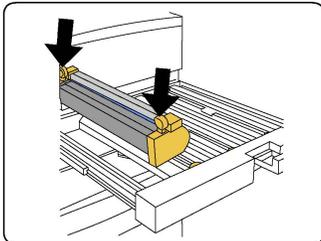
10. Press both ends of the drum cartridge to place it in a horizontal position.
