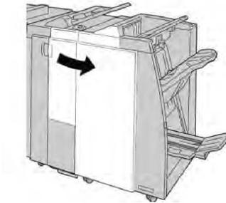
3. Move the levers **3b** and **3d**; remove the jammed paper.
