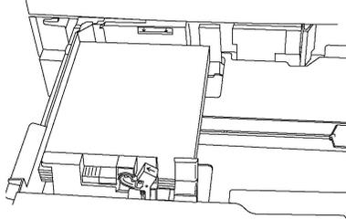
5. Adjust the guides so they touch the edges of the stack.
