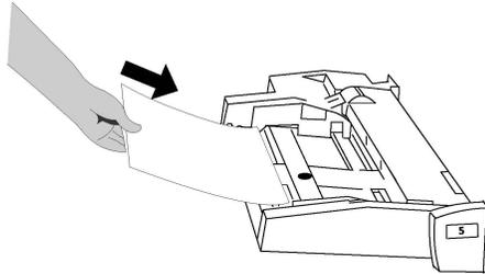
4. Adjust the width guides until they just touch the edges of the stack.
