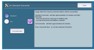
A *Full Overwrite* takes approximately 60 minutes and includes all data. Select the *Overwrite* option required and select **Overwrite Now** to run the overwrite process.
