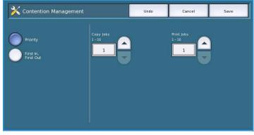
• **First In, First Out** instructs the device to process jobs based on when they are received. The jobs are processed in the order they enter the job list.
