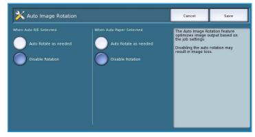
• Use the **When Auto Paper Selected** options to instruct the system how to proceed if *Auto Paper* is selected. Select **Auto Rotate as needed** to allow automatic rotation, or **Disable Rotation** to restrict the device from rotating the image.
