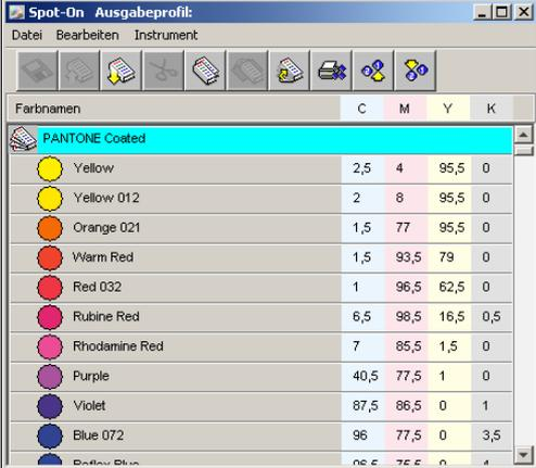
The screenshot shows the 'Spot-On' software window with the 'Ausgabeprofil' (Output Profile) set to 'PANTONE Coated'. The interface includes a menu bar with 'Datei', 'Bearbeiten', and 'Instrument'. Below the menu is a toolbar with various icons. The main area displays a list of color groups with their corresponding CMYK values. The 'PANTONE Coated' group is highlighted in blue.
