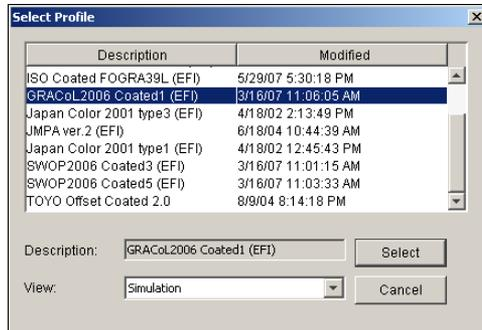
Simulation lists the simulation profiles resident on the EX8002. Output lists the output profiles resident on the EX8002.
