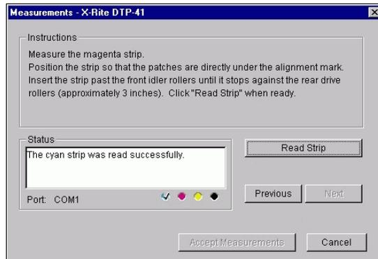
A check mark appears on the circle of the color just read, and the Status field indicates the color was measured successfully.
