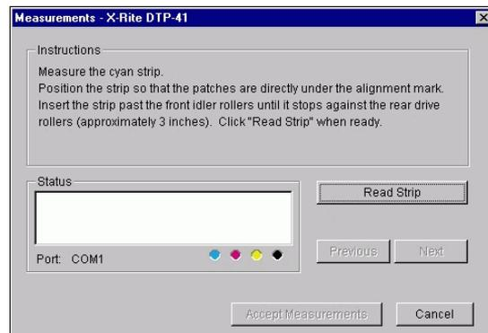
Align the page in the measurement page slot of the DTP41 so that the appropriate color column is centered below the alignment mark. Insert the page about three inches, past the front idler rollers, until it rests against the rear drive rollers and you feel resistance.
