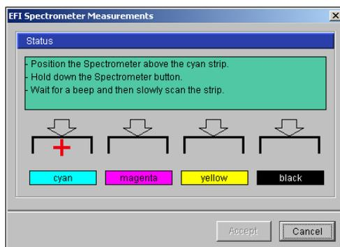
**11 For a more accurate measurement, place several sheets of plain white paper beneath the Measurement Page.**
