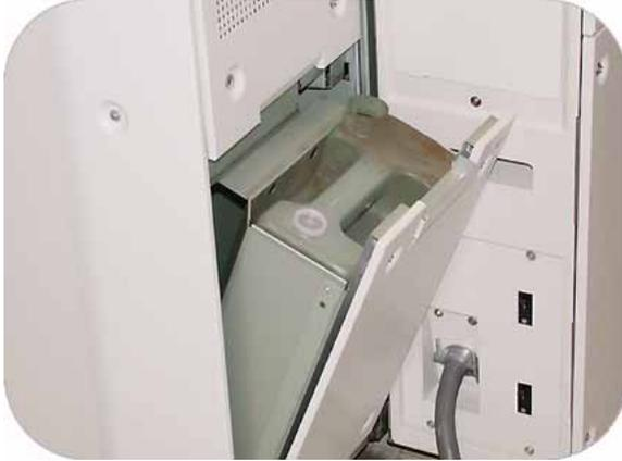
2. Install the cap (found on the side of the bottle) and dispose of the bottle in accordance to local regulations.
