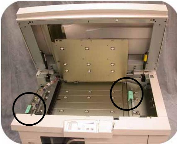
3. Lift the green handle, or handles, indicated on the UI and remove all paper in the Bypass area. Remove paper only from the areas indicated.
