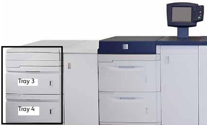
The Second Feeder Module (SFM) is an optional feeding device that contains Trays 3 and 4. This module holds the same number and types of Media as Trays 1 and 2.
