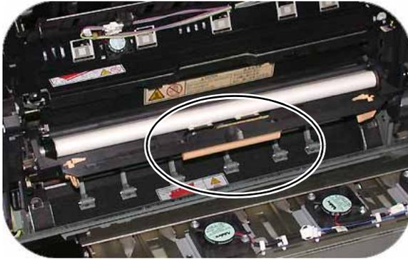
5. Align the yellow tabs on the sides of the Fuser Web with the yellow marker on each rail and slide the web all the way into the fuser.
