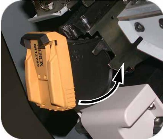
6. Push the Cartridge in to the Stapler Unit.
