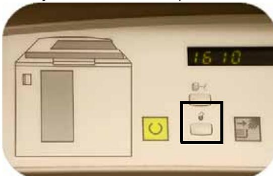
2. Open the front door when the Unload Light illuminates.
