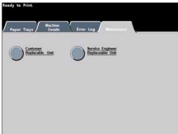
The Customer Replaceable Unit screen displays a gauge or a check mark indicating the level at which the consumable is.
