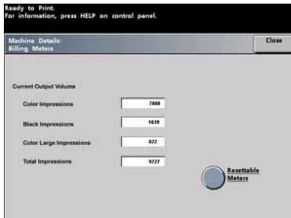
To reset the meters to zero, touch the **Resettable Meters** button. On the following screen touch the **Reset** button.
