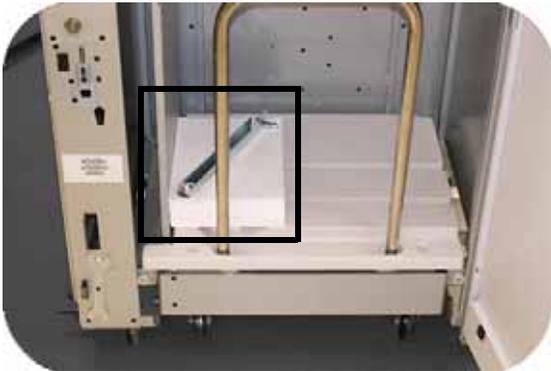
4. Pull the Stacker Cart straight out. Remove the securing bar.
