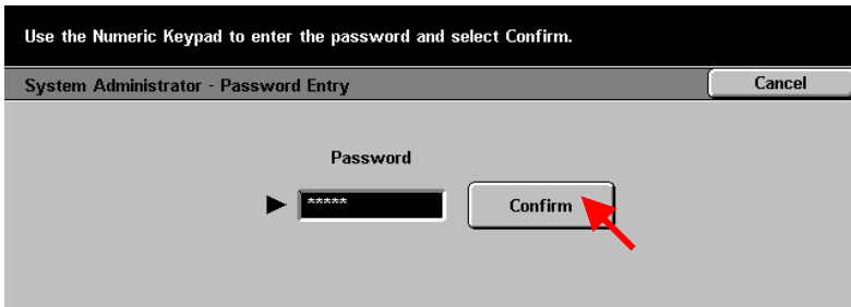
Fig. 2 Enter the System Administrator Password from the Numeric Keypad and then press Confirm . (See Machine Administration User Guide for default password)
