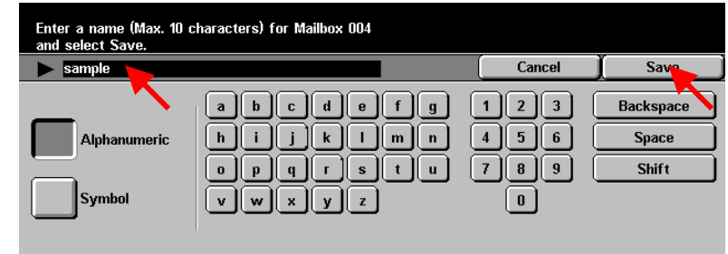
Fig. 9 Enter the name for the Mailbox using the keyboard displayed. The mailbox name may be up to 10 characters. Press Save after entering the name.
