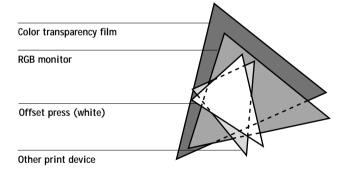
You need to account for the gamut of your print device when designing on a color monitor. When printed, colors that fall outside the print device's gamut are "mapped" to printable colors. This process, referred to as **gamut mapping**, takes place when color data is converted or adjusted to meet the color space and gamut requirements of a print device.
