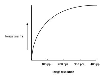
Raster images prepared for offset printing may need to be at higher resolutions than needed for proofing on your DocuColor 40 CP. Check with your prepress service provider and printing vendor for their recommendations on image resolution based on your job specifications.
