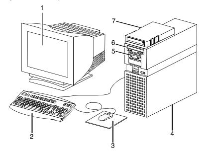
Figure 2-3. Components of the Sun Ultra 60 workstation
