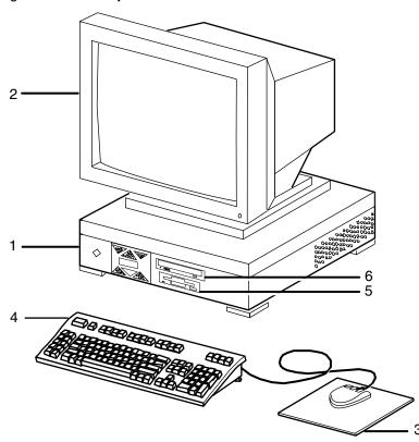
Figure 2-1. Components of the Sun Ultra 2 workstation
