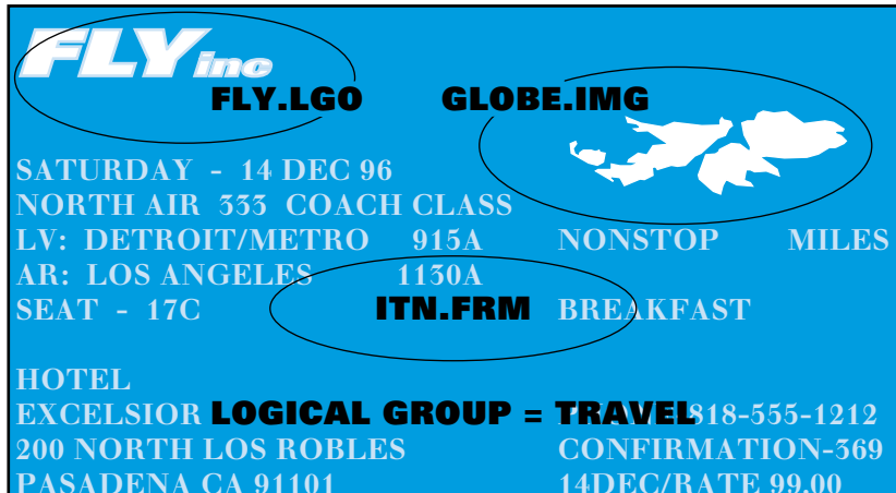
FIGURE 8. Use the logical group attribute to organize multiple printer resources by a single name.
