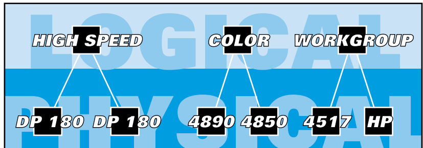
FIGURE 5. Balance the workload among printers and simplify job submission using logical printers.
