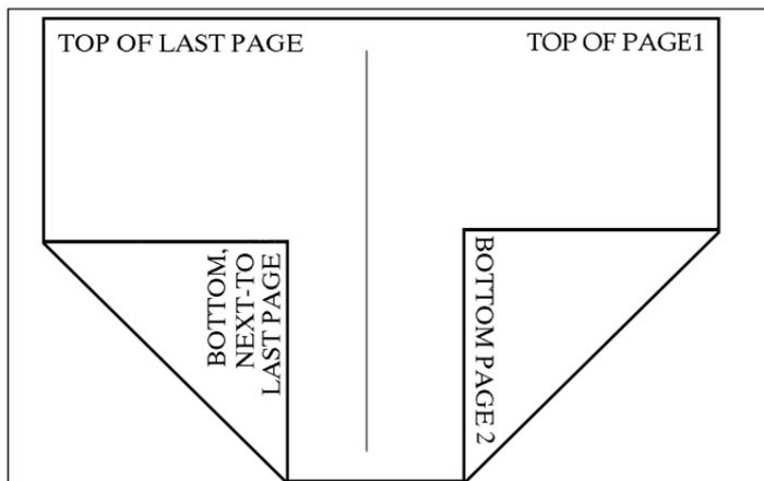
Figure 3-3. 2-UP, rotate, and collated output
