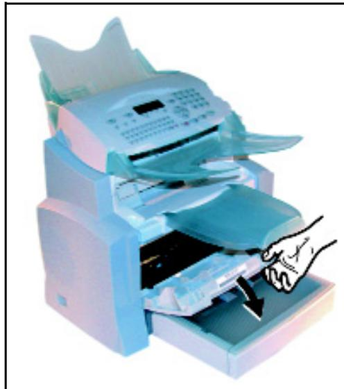
**CAUTION:** The fusing unit located inside the printer may become very hot during operation. To avoid injury - do not touch.
