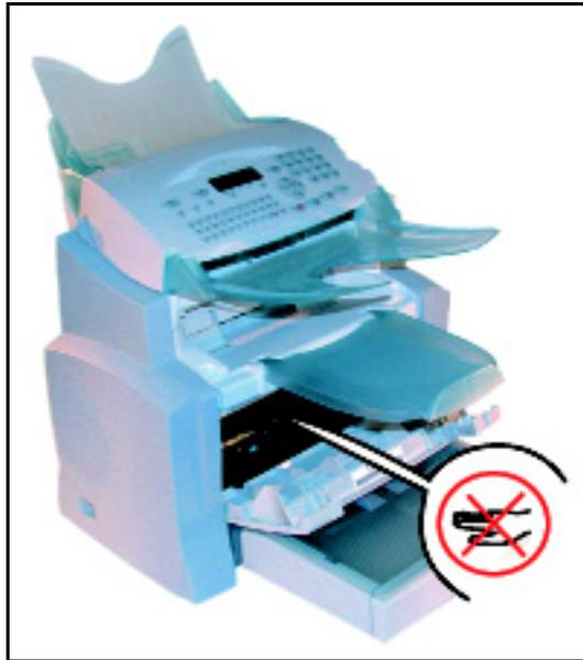
**CAUTION:** The fusing unit located inside and at the bottom of the printer may become very hot during operation. To avoid injury - do not touch.
