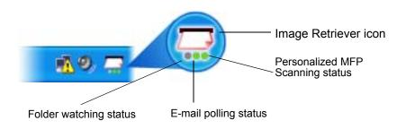
The icon has three indicator lights at the bottom. They represent the status of e-mail polling, folder watching and Personalized MFP Scanning by means of different colors: dark green - monitoring; light green - processing; grey - inactive; red - error.
