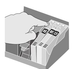
Click the **Change** button. A window opens, prompting you to select the item you are installing. Choose a color ink cartridge. Click **OK**. Open the printer cover. The print head moves to the center of the printer.
