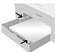
Remove any other media and place up to 30 transparencies in Tray 1 with the rough side down. If your transparency has an adhesive strip you can peel it off after printing. You can print with the adhesive strip facing either way.
