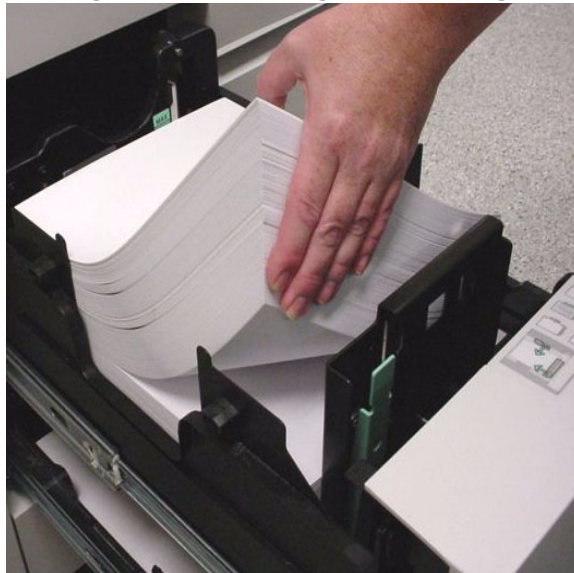
Figure 2-5. Fanning the lead edge
