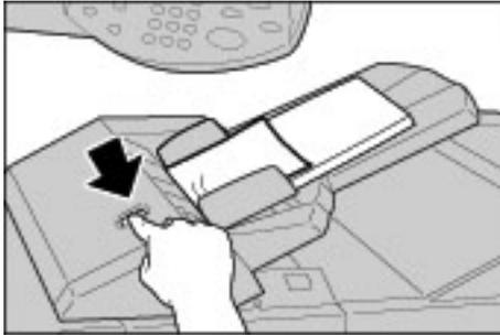
2. Open cover 1e and then remove the jammed paper and all paper loaded in the Post-Process Inserter.
