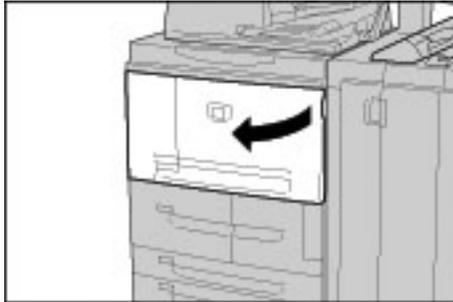
2. Open the Waste Toner Container cover and push the lever down.
