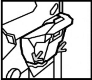
7. Move the lever to the left; the lock position.
