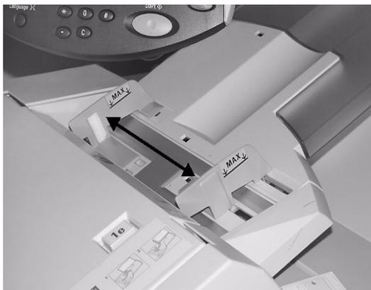
2. If the paper is preprinted, load the paper with the printed side facing up and with the tab side to be fed first.
