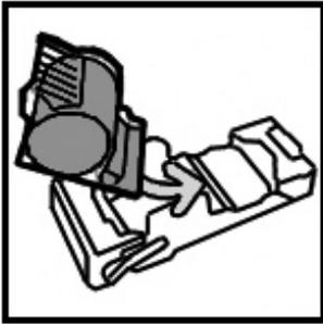
5. Push the removed cartridge back to the original position until it clicks into place.
