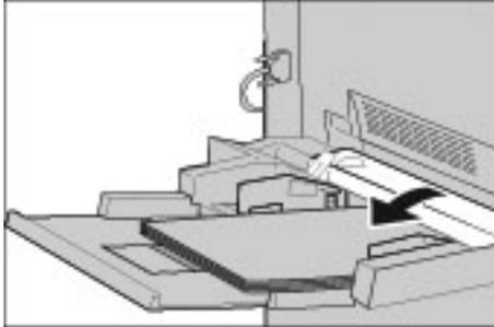
2. Remove the jammed paper and all paper loaded in paper Tray 5 (Bypass).
