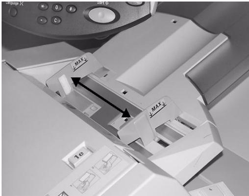
2. Load the paper, aligning to the front side of the tray. If the paper is preprinted, load the paper with the printed side facing up and with the tab side to be fed first.
