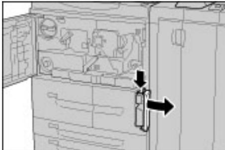
3. Grasp the handle of the Waste Toner Container with one hand, and pull it out of the machine about half way.
