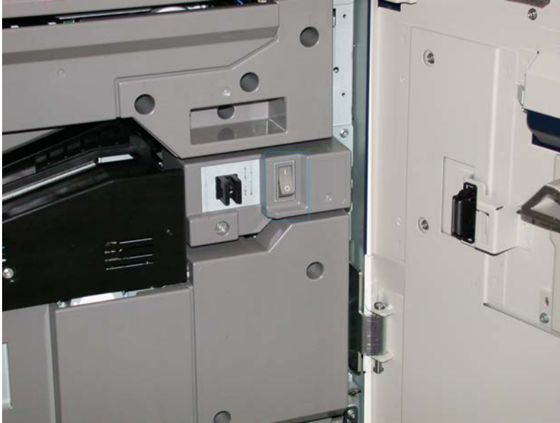
Figure 2. The Power On/Off Button (On top of the Press)
