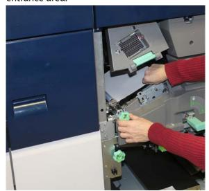
**4.** Rotate the **5d** knob clockwise to advance paper and pull down on the **5c** green lever to remove any paper in this area.
