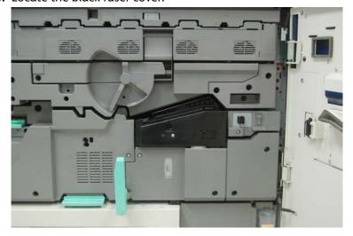
**4.** Remove the fuser cover by using the T10 Torx driver to unscrew the one mounting screw at the center of the cover.
