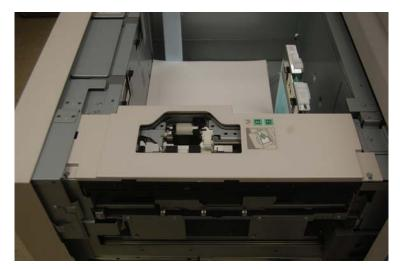
3. Remove the nudger roll by pushing down on the black tab with one hand (which raises the roll upward) and then squeezing the metal shaft on both ends with your other hand. Lift out the nudger roll.
