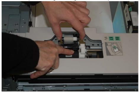
5. Remove and replace the retard roll using the same technique.
