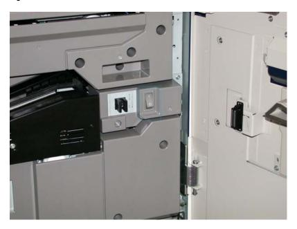
Figure 2. The Power On/Off Button (On top of the Press)
