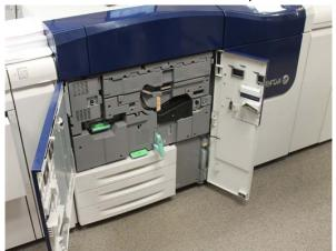
**3.** Locate the green Handle (2) and rotate clockwise to the horizontal position to unlock the Transfer Drawer.
