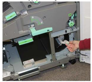
**6.** It is now safe to unlock and pull out the Exit Module Drawer. Grasp the green Drawer handle (4) and rotate handle to the right to the horizontal position. Slowly pull out the Drawer assembly until it stops.
