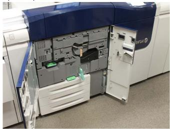
3. Rotate and turn the R1-R4 Drum Drawer Handle to the unlock position.
