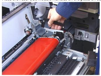
**12.** Facing the right side of the drawer, push the module slightly away from you and lift the Fuser Belt straight up and out of the press, letting the weight of the module hang in your hands.
