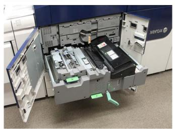
**4.** Locate and lift up the green **2b** lever to remove jammed paper from the registration area.
