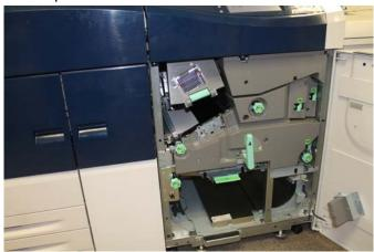
3. To clear the entrance baffle area (3a and 3b), lift the Upper Cooling 3a lever and also rotate the 3b knob clockwise to advance the paper jammed in the Module Entrance Roll. Ensure paper has completely moved through the roll beyond the entrance area.
