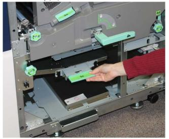
5. At the far right of the press, locate the 5a lever and 5b knob. Pull down on the 5a lever to access the inverter area and remove any paper. Rotate the 5b knob clockwise to advance any paper coming down into the inverter.
