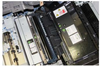
7. Locate and push down on the green **2f** lever to remove jammed paper from the Duplex Transport Baffle.
