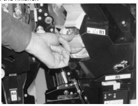
**4.** Hold the positions as indicated by the arrow and remove the staple cartridge from the unit.
