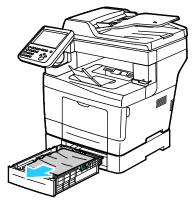
3. Remove any paper jammed at the front of the printer.
