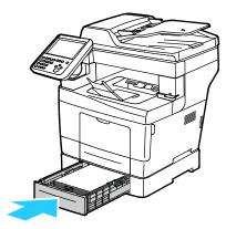
Note: If the tray is extended for legal size paper, the tray protrudes when it is inserted into the printer.
