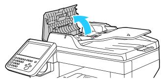
2. With a clean, lint-free cloth moistened with water, wipe the feed rollers and the separation pad until they are clean.
