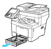
3. To extend the tray, with one hand, hold the back of the tray. With the other hand, at the front of the tray, press the release latch and pull the ends outward until they latch.
