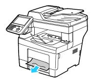
6. Insert tray 1 into the printer, then push it in all the way.
