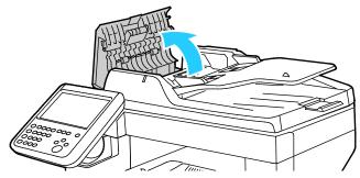
3. If the paper is jammed in the exit of the duplex automatic document feeder, pull it out as illustrated.
