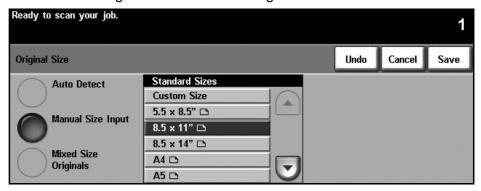
**Auto Detect:** Use this option to allow the machine to automatically recognize the size of the originals being fed through the document feeder.
