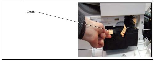
**5.** Squeeze the retaining clip and remove the used SMart Kit<sup>TM</sup> Drum Cartridge.
