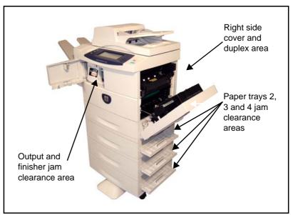
1. Open the machine covers and use the green handles and knobs indicated in the instructions displayed to remove the jammed paper.
