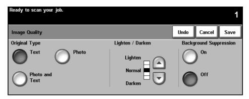
The **Original Type** option is used to enhance the copy quality of the output based on the type of original being scanned.
