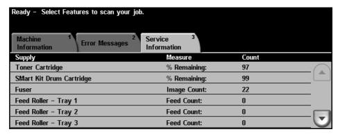
The Services Information tab displays the current status of customer replaceable and engineer replaceable consumables
