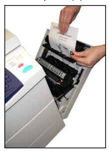
2. Ensure that all jam clearance handles and levers are returned to their correct positions.
