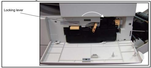
4. Lift the latch to release the toner cartridge and remove the used toner cartridge.
