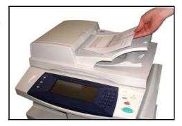
Up to 50 sheets of 20 lb (80 g/m²) bond paper can be loaded. Weight ranges from 12 lb to 28 lb (50 - 120 g/m²) - refer to Electrical Specifications in the Specifications chapter on page 166 for full Document Feeder Specifications.
