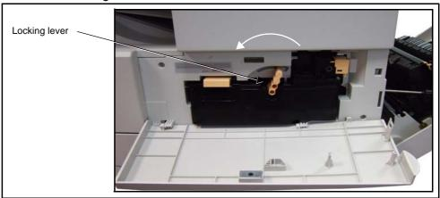
4. Lift the latch to release the toner cartridge and remove the toner cartridge.
