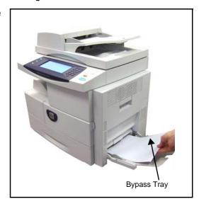
4. Adjust the paper guide to the width of the stack of print material. Ensure you have not loaded too much print media. The stack should be under the Max. Fill Line.
