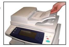
Up to 50 sheets of 20 lb (80 g/m²) bond paper can be loaded. Weight ranges from 12 lb to 28 lb (50 - 120 g/m²) - refer to Electrical Specifications in the Specifications chapter on page 166 for full Document Feeder Specifications.
