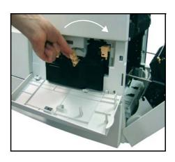
If after fitting a new toner cartridge the front door will not close, check that the toner cartridge is positioned and latched correctly.
