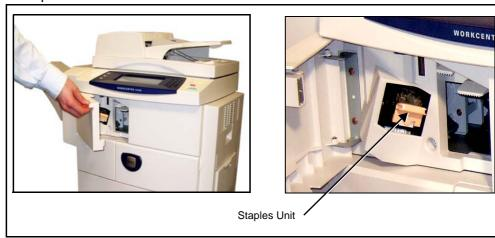
2. Use the latch to pull out the staples unit. Remove the staples unit.
