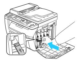
10. Align the black toner cartridge with the rear toner slot. Press firmly near the center of the cartridge until it clicks into place.
