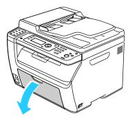
2. Place the paper cover on the main tray and align the tabs with the marks on the tray.
