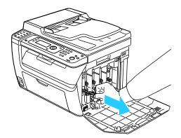
7. Insert the cleaning rod into the hole indicated by the arrow in the middle of the toner cartridge slot. Push in the cleaning rod until it stops, then pull it out.
