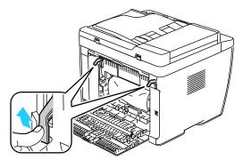
3. Remove any jammed paper from the back of the printer.
