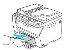
3. Remove any paper jammed at the front of the printer.
