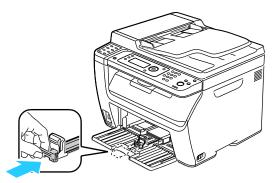
9. Place the bypass tray on the main tray, then align the tabs with the marks.
