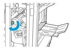
3. Remove the jammed paper by pulling in the direction shown.
