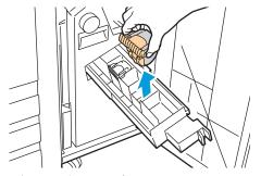
6. Push the staple cartridge into the staple cartridge unit.
