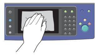
Use a lightly dampened cloth to clean the outside of the document feeder, output trays, paper trays, and outside areas of your printer.
