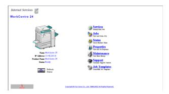
Internet Services are a series of web pages located within the machine network communication settings to be conveniently configured from a web browser running on a remotely located workstation.
