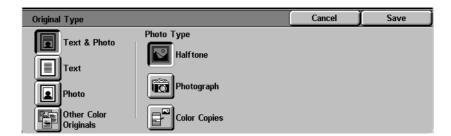
The Original Type feature enables you to define the kind of original document you wish to copy. The copier automatically makes adjustments to optimize the copy based on the original type.
