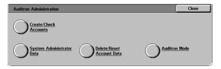
Auditron is an audit feature. This feature electronically records the number of copies or prints made for each user account and controls the access and use of the printer/copier.
