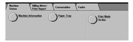
Machine status can be checked by selecting the Machine Status button on the Control Panel. The following items are on the *Machine Status* screen:
