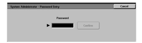
2 Enter the password using the numeric keypad on the Control Panel, and select **Confirm**. The *System Administrator Menu* screen is displayed.
