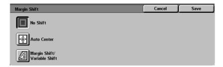
The Margin Shift feature allows you to shift the position of the image on the copy. The image can be centered on the copy or moved to the top, bottom, left or right. When copying both sides, different settings can be set for Side 1 and Side 2.
