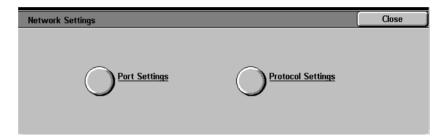
Network Settings consists of Port Setting, which determines the type of interface of the main unit that is connected to clients, and Protocol Setting, which determines the necessary condition for the communication.
