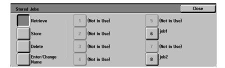
The Stored Jobs feature allows you to program various feature settings in the built-in copier memory as a single job. Up to 8 jobs can be stored and up to 18 characters can be entered for each job name. This feature is especially helpful for complex jobs that you run frequently.
