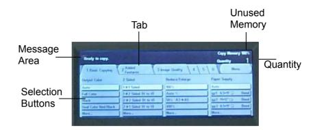
Press the buttons and tabs displayed in the Touch Screen to select features or respond to on screen instructions. The selected buttons are highlighted to indicate activation. Buttons that do not have three-dimensional shadows are not active, and cannot be selected.
