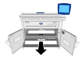
3. Remove the Media Shaft and the partial roll or core from the machine.
