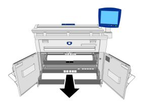
3. Press the Cutter Button to cut the lead edge of the media.
