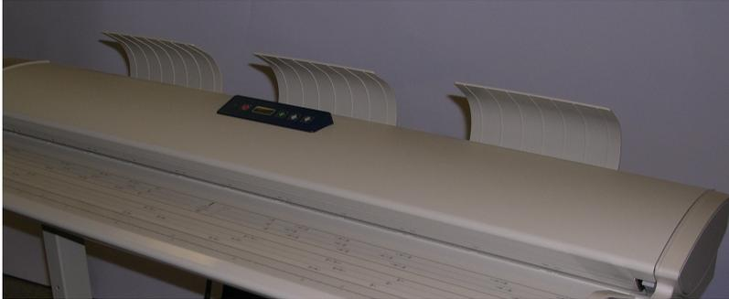
Insert each of the three Media Exit Deflectors into the corresponding slots along the upper edge of the rear of the scanner. Ensure that they are inserted fully into the slots and that they do not block the document exit opening. This is easy to overlook when installing them.
