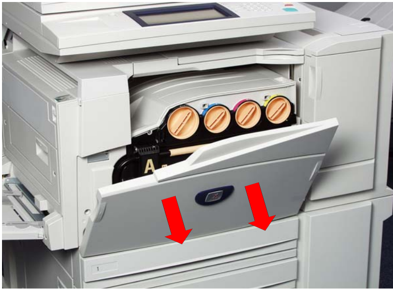
Fig. 1 Make sure that the machine has stopped before opening the front cover.
