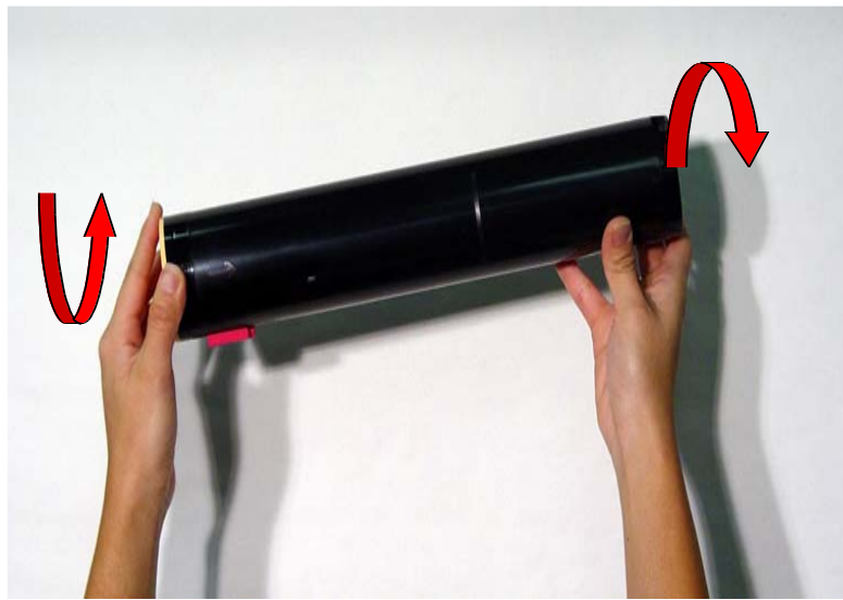
Fig. 4 Lightly shake the new toner cartridge three or four times up and down to the left and right.
