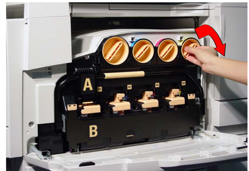
Fig. 6 Turn the toner cartridge to the right down to the key (closed).
