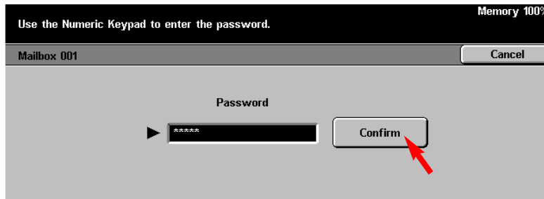
Fig. 6 Enter the Password for the mailbox using the numeric keypad and press Confirm . (If the password option was not selected proceed to the next step.)
