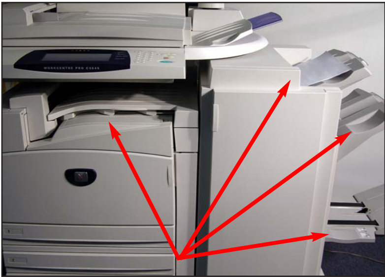
Fig. 10 Depending on the machine configuration and features selection the job will be delivered to one of the output trays available.
