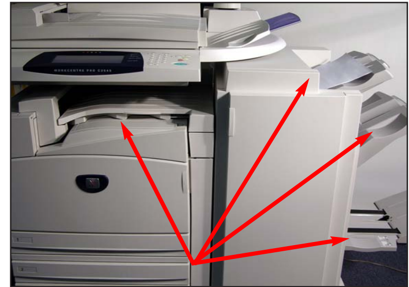
Fig. 2-7 Depending on the machine configuration and features selection the job will be delivered to one of the output trays available.
