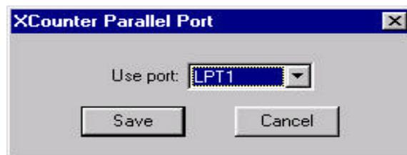
The XCounter parallel port monitor prints to local LPT ports. However, the XCounter parallel port monitor cannot share an LPT port with the default NT Local Port monitor, so ensure that no printers have been assigned to the LPT port that are required to use with XCounter. If no ports are available, the error message "All parallel ports are already in use" will be displayed.
