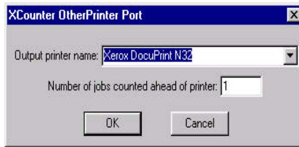
The XCounter OtherPrinter port sends jobs to other print queues. The OtherPrinter port cannot print to remote Windows printer shares - the queue must be located on the same NT printer host.
