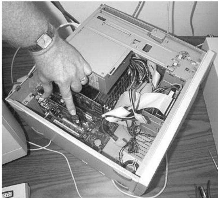
**Inserting the FireBoard into the PC.**
