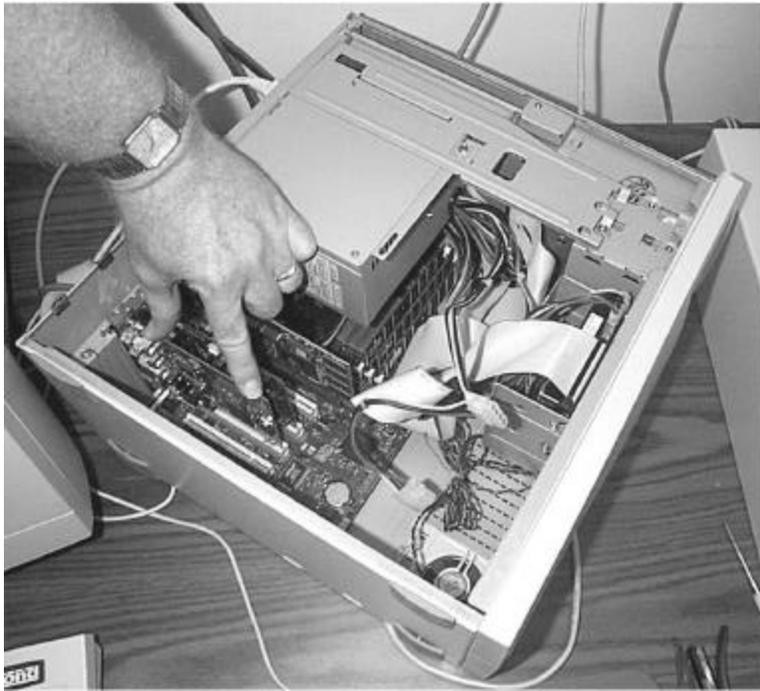
**Inserting the IEEE1394 Board into the PC.**
