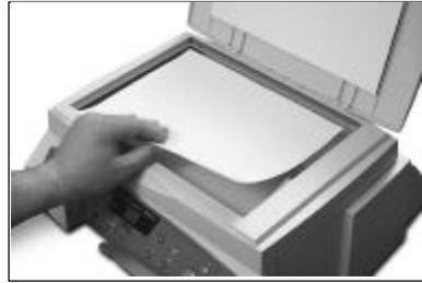
*NOTE: If the scanning process does not begin, try lowering the resolution rate in the tab menu, and repeat the scan step.*
