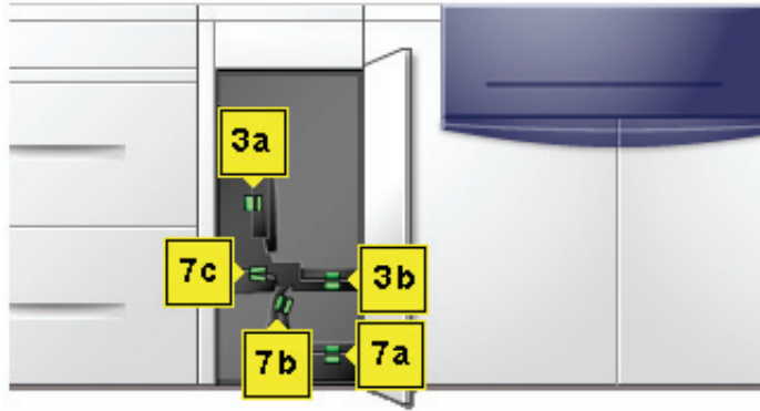
Transport Module Jam Clearance Areas
