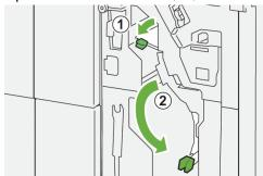
b) Rotate knob **1b** clockwise ( $^{\textcircled{1}}$ ) and remove the jammed paper ( $^{\textcircled{2}}$ ).
