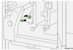
d) Use the poker to sweep any remaining waste or debris from inside the trimmer into the trimmer waste container.
