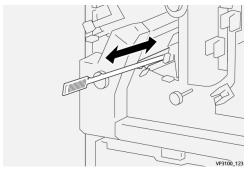
e) you have difficulty sweeping waste into the trimmer waste container, use the poker to gather waste, and then remove the waste by hand.
