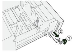
**5.** Install the Postcard bracket so that it sits on the locating pins on the upper frame and in the grooves on the bottom of the tray.
