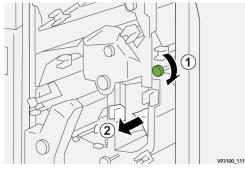
**4.** Rotate knob **2f** counterclockwise ( $^{\textcircled{1}}$ ) and remove jammed paper ( $^{\textcircled{2}}$ ).
