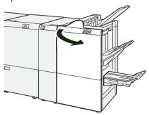
**2.** Open lever  $\mathbf{1a}$  to the left (1) and remove the jammed paper (2).
