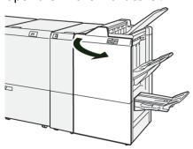
**2.** Open lever 3a to the left (1) and remove the jammed paper (2).
