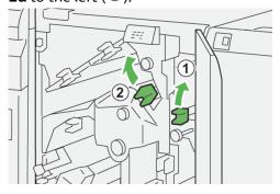
7. Rotate knob **2b** counterclockwise ( $^{\textcircled{1}}$ ) and remove jammed papers ( $^{\textcircled{2}}$ ).
