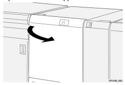
**2.** Open lever **3a** to the right ( $^{\textcircled{1}}$ ), lever **4b** downward ( $^{\textcircled{2}}$ ) and lever **4c** to the right ( $^{\textcircled{3}}$ ). Remove jammed paper ( $^{\textcircled{4}}$ ).
