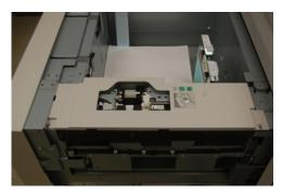
3. Remove the nudger roll by pushing down on the black tab with one hand (which raises the roll upward) and then squeezing the metal shaft on both ends with your other hand. Lift out the nudger roll.
