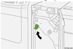
**4.** If you encounter difficulty when removing jammed paper, open lever 1c upward 1c and carefully remove jammed paper 2c.
