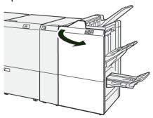
**2.** Open lever **1c** to the right ( $^{\textcircled{1}}$ ) and rotate knob **1e** clockwise ( $^{\textcircled{2}}$ ). Remove the jammed paper ( $^{\textcircled{3}}$ ).
