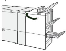
**2.** Open lever **1d** to the right ( $^{\textcircled{1}}$ ) and rotate knob **1e** clockwise ( $^{\textcircled{2}}$ ). Remove the jammed paper ( $^{\textcircled{3}}$ ).
