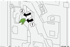
3. If you have difficulty removing paper jam, pull out the Saddle Stitch Unit 3  $(^{\textcircled{1}})$  and remove the jammed paper  $(^{\textcircled{2}})$ .
