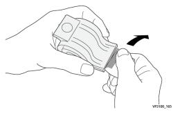
7. Insert the staple cartridge into the unit.
