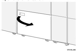
b) Remove the supplied poker (stick) from its location inside the lower cover.
