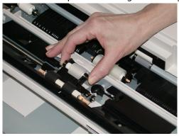
5. Remove and replace the retard roll using the same technique.
