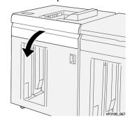
**2.** Open lever **2a** downward ( $^{\textcircled{1}}$ ) and remove jammed papers( $^{\textcircled{2}}$ ).
