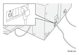
The circuit breaker is located on the rear of the device. The circuit breaker is normally in the **ON** position.
