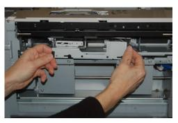
7. With the retard assembly out, access and remove the feed roll. To remove, squeeze both ends of the metal shaft and lift out. To replace, squeeze both ends of the new roll shaft, and insert and release the roll ends into the notches.
