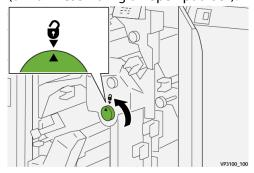
3. Open lever **2c** downward ( $^{\textcircled{1}}$ ) and remove jammed paper ( $^{\textcircled{2}}$ ).
