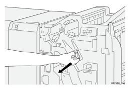
3. Open the unit cover, and remove the jammed staples.
