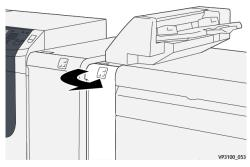
**2.** Open lever  $\mathbf{1a}$  upward  $\mathbf{1}$  and turn knob  $\mathbf{1b}$  counterclockwise  $\mathbf{2}$ . Remove any jammed paper  $\mathbf{3}$ .
