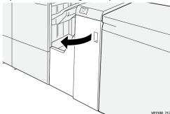
2. Open lever 1 downward and remove the jammed paper.
