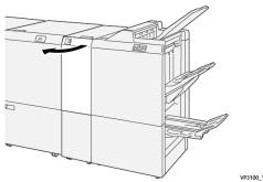
**2.** Open lever **2a** upward ( $^{\textcircled{1}}$ ) and lever **2b** to the left ( $^{\textcircled{2}}$ ). Remove jammed paper ( $^{\textcircled{3}}$ ).
