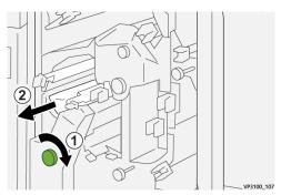
**4.** If you have difficulty removing the jammed sheet, grasp the top edge at the inner-right side of the sheet, and gently pull out the sheet to remove it.
