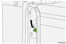
**4.** If you have difficulty when removing jammed paper, open lever **1c** to the right  $\bigcirc$  and turn knob **1b** counterclockwise  $\bigcirc$ . Remove any jammed paper  $\bigcirc$ 3.
