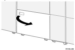
2. Pull out and remove the waste container.
