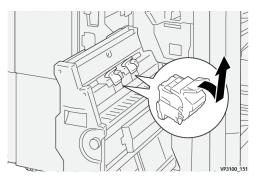
4. While holding the tabs on the new staple cartridge, push in the cartridge until it seats.
