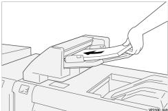
If the paper is preprinted, load the paper with the printed side facing up.
