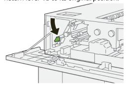
**5.** Open lever **2a** downward ( $^{\textcircled{1}}$ ) and remove jammed paper ( $^{\textcircled{2}}$ ).
