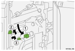
**3.** Rotate knob **2f** clockwise ( $^{\textcircled{1}}$ ) and remove jammed paper ( $^{\textcircled{2}}$ ).
