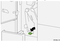
7. Close the trifold output tray 2d by pushing it in completely.
