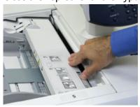
**5.** Pull open the **Top Drawer** (located at the top of Trays 6 and 7).
