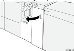
**2.** Open lever **2** to the right  $(^{\textcircled{1}})$  and rotate the knob counterclockwise  $(^{\textcircled{2}})$ . Remove the jammed paper.
