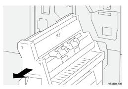
3. Rotate knob 3b counterclockwise (1) and remove the jammed paper (2).
