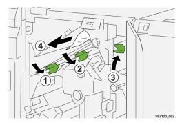
**3.** If you have difficulty removing any paper jams, rotate knob **1c** clockwise ( $^{\textcircled{1}}$ ), and remove the jammed paper ( $^{\textcircled{2}}$ ).
