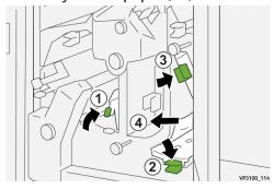
3. Rotate knob  $\mathbf{4d}$  counterclockwise (1) and remove jammed paper (2).
