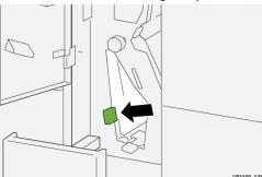
**5.** If you have difficulty removing any paper jams, open lever **2f** to the right  $(^{\textcircled{1}})$  and rotate knob **2c** counterclockwise  $(^{\textcircled{2}})$ . Remove jammed paper  $(^{\textcircled{3}})$ .
