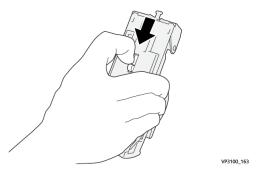
**5.** Turn the unit up while holding the lever, and then take out the staple cartridge from the unit.
