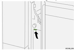
**4.** If you have difficulty when removing jammed paper, open lever **1a** upward ① and turn knob **1e** counterclockwise ②. Remove any jammed paper ②.
