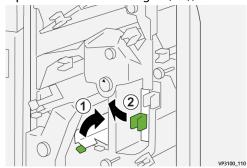
**3.** Rotate knob **3c** clockwise (1) and remove jammed paper (2).
