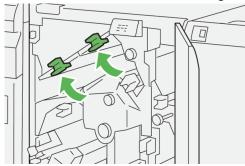
**6.** If you have difficulty removing any paper jams, open lever 1d upward (1) and lever 2a to the left (2).
