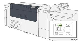
The following occurs when there is an fault, such as paper jams, open doors or covers, or a press malfunction:
