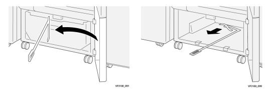
**5.** Return the poker to its original position on the inside of the lower cover.
