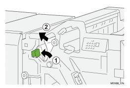
**3.** If you have difficulty removing any paper jams, rotate knob **1b** clockwise ( $^{\textcircled{1}}$ ) and remove the jammed paper ( $^{\textcircled{2}}$ ).
