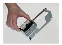
10. Reinstall the retard assembly into the tray. Align the cutout holes of the assembly with the frame of the tray so the pin holes match up. Insert the assembly into the frame. Slide the assembly all the way to the right using the pin as a guideline. Ensure the device is all the way into the slots and the 3 screw areas align.
