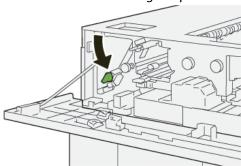
**4.** Open lever **2b** upward (1) and turn knob **2c** counterclockwise (2); remove jammed papers (3).
