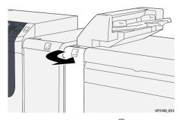
2. Open lever **1d** downward ① and turn knob **1e** counterclockwise ②. Remove any jammed paper ③.
