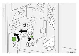
**5.** Rotate knob **3c** clockwise (1) and remove jammed paper (2).
