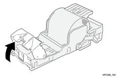
4. Locate the lever on the back of the unit.
