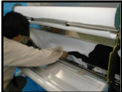
2. Carefully remove the jammed media from the cutter unit.
