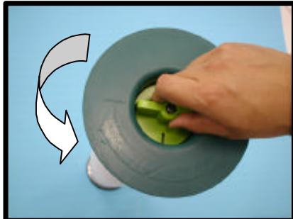
2. Rotate the end cap rearward to rewind the media onto the media roll.
