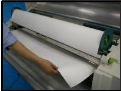
3. If the media is protruding from the media exit, cut that portion of the media using scissors or a knife.
