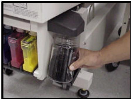
4. Set the new waste ink bottle on the waste ink bottle tray. Ensure that the bottle is properly seated on the tray before continuing.
