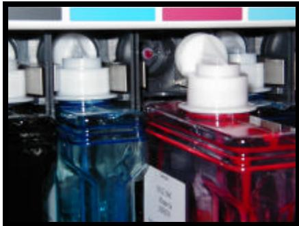
5. Ensure that the waste ink bottle is in place and properly seated.
