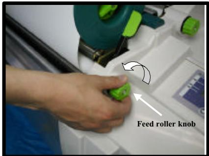
11. Rotate the feed roller knob toward you. Continue to forward the media until you hear a beep from the printer. The printer will sense the new media's leading edge. Ensure that there is even tension and no wrinkles on the media.
