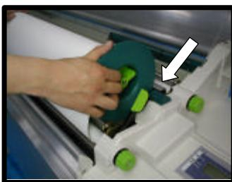
8. Set the right end cap at the position matching the media width. The front guides are freely-rotating support rollers.
