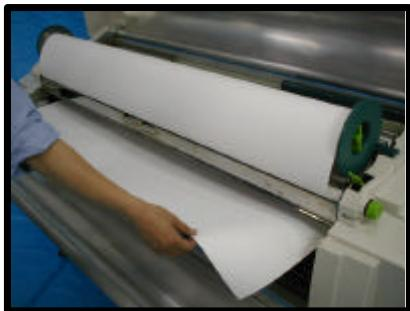
3. If the jam occurred before the media was ejected from the media exit, pull out the media for easy cutting.
