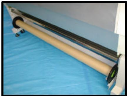
3. Set the FLANGE on the plastic roller bearing on the right side.
