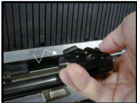
9. Tilt and slide the cutter blade from the cutter holder.
