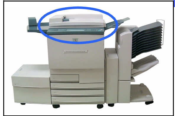
Figure 1: Document Centre ColorSeries 50 with a Duplex Automatic Document Feeder
