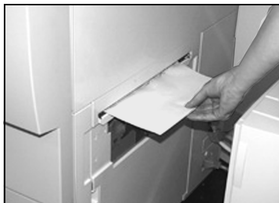
Figure 3: Removing paper from the interface area
