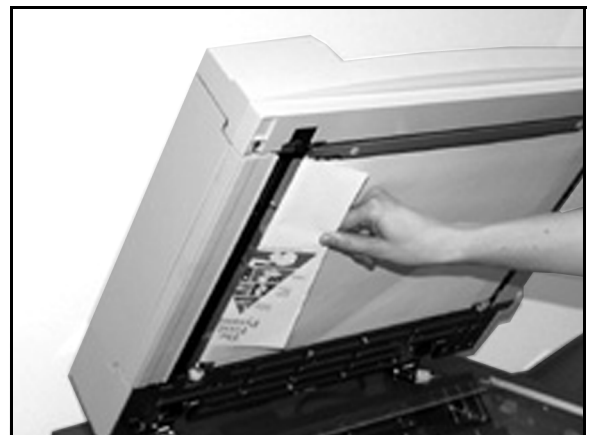
Figure 10: Removing jammed paper
