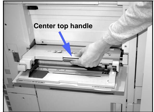
Figure 16: Grasping the top of Paper Tray 5
