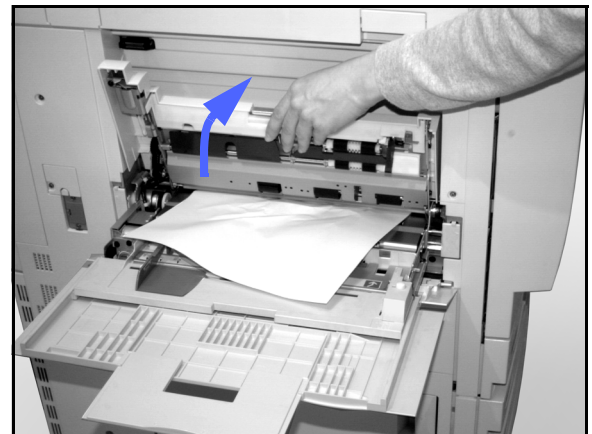
Figure 17: Lifting the top of Paper Tray 5
