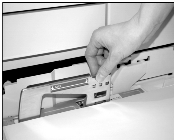
Figure 7: Adjusting the Rear Paper Guide
