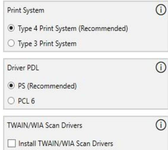
The image shows three panels of installation options. The first panel, 'Print System', has 'Type 4 Print System (Recommended)' selected with a radio button, and 'Type 3 Print System' is unselected. The second panel, 'Driver PDL', has 'PS (Recommended)' selected with a radio button, and 'PCL 6' is unselected. The third panel, 'TWAIN/WIA Scan Drivers', has an unchecked checkbox for 'Install TWAIN/WIA Scan Drivers'. Each panel has an information icon (i) in the top right corner.
