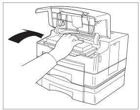
**8** Reinstall the Printer Cartridge and close the top door.
