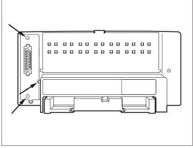
Unscrew the three screws securing the system controller board and discard the metal plate.
