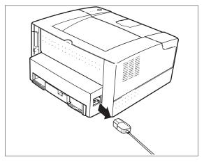
1 Remove the power cord from the printer power receptacle.
