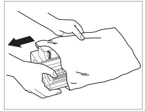
**2** Remove the Printer Cartridge from its packaging.
