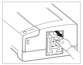
**3** Remove the screw and the metal cover.
