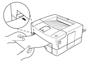
Figure 4.6 Using the Manual Feed
