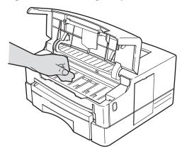
Before cleaning the printer, disconnect the printer from its power source.
