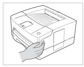
1 Press the top door release button to open the top door.
