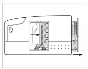
**7** Slide the system controller out of the printer and put it on a flat surface.
