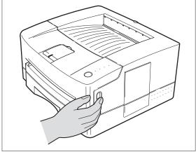
2 Press the top door release button to open the top door.
