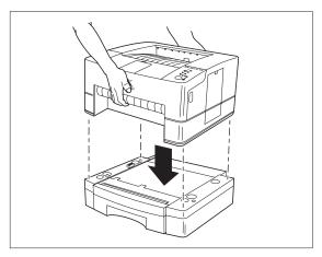
5 Lift the printer and place it on top of the Lower Base, as shown.
