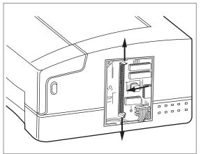
If the controller has an additional SIMM installed, remove it.
