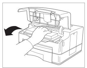
**3** Remove the Printer Cartridge from the printer and close the top door.
