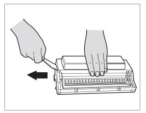
Remove the Plastic Strip from the Printer Cartridge.
