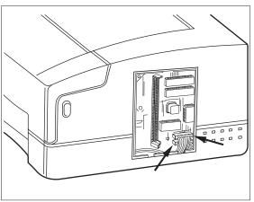
**4** Disconnect the two ribbon cable connectors from the controller.
