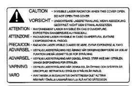
CAUTION: Avoid exposure to invisible laser radiation when the development unit is not installed.
