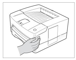
**7** Press the top door release button to open the top door.
