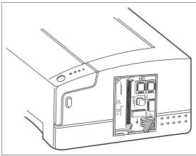
**4** Locate the SIMM slot on the system controller board.
