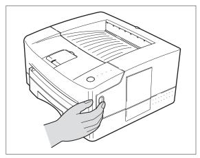
Press the top door release button to open the top door.
