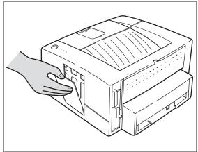
2 Remove the panel cover on the right side by pushing the latch down and pulling it out and up.
