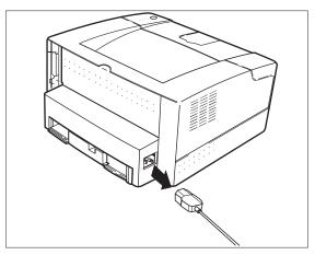
1 Remove the power cord from the printer power receptacle.
