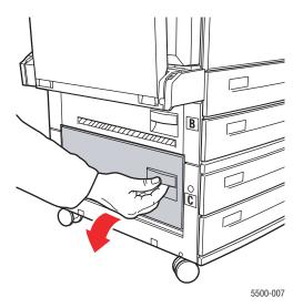
**3.** Pull the jammed paper out of the printer. Confirm that all paper fragments are removed.
