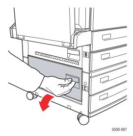
**6.** Pull the jammed paper out of the printer. Confirm that all paper fragments are removed.
