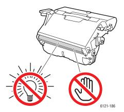
3. Place the removed imaging unit aside, laying it horizontally as shown in the picture at right. Be sure to keep the imaging unit horizontal and place it where it will not become dirty. Do not leave the imaging unit removed for more than 15 minutes, and do not place it in a location where it would be exposed to direct light, such as sunlight.
