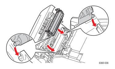
• Lock the transfer roller into the printer by pushing down on the tabs until you hear a click.
