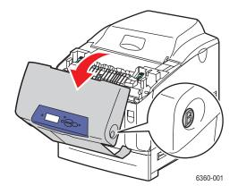
**2.** Pull up the two levers at both ends of the fuser.
