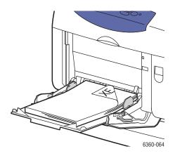
• For **2-sided printing**, place the first side to be printed **faceup** with the **bottom** of the page entering the printer first.
