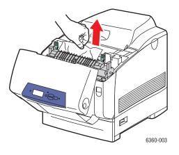
4. Completely push down the two levers at both ends of the fuser.
