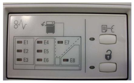
3. After the HCS stacker door is closed, press the **Interrupt** button again on the Xerox 700 digital color press, and the job resumes printing.
