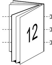
**Perfect binding:** In Perfect binding, the signatures are folded individually, and then stacked together along common edge, which is flattened and glued to form the spine of the booklet.
