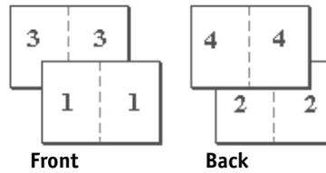
**Gang-Up - Cut & stack:** Choose this setting to speed print a job so that when the sheets are stacked and cut from the central position, the job is numbered in order and separated as two stacks. The order of print is such that when they are cut in half, they can be combined to form a single complete set of the document, in faster printing time.
