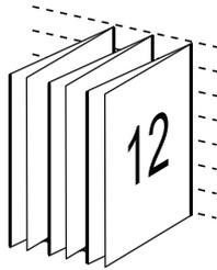
**Nested Saddle:** The Nested Saddle binding method combines saddle and perfect binding methods by stacking two or more saddles (also called “groups” or “subsets”) together along the common fold, then glued together at the fold to form the spine of the booklet.
