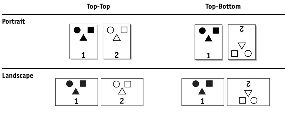
For Top-Top manual duplexing, keep the pages oriented in the same direction as they arrive in the output tray, except face down. For example, if the image is upside down and the pages are face up, load them with the image upside down and the pages face down.
