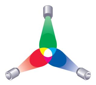
A familiar device that is based on this color model is the computer monitor, illustrated in the following figure. Monitors have red, green, and blue **phosphors** that emit varying amounts of light to display a given color. Scanners create digital representations of colors by measuring their red, green, and blue components through colored filters.
