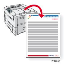
All the printable pages have this format, with color bars at the top and at the bottom of the page. Print these pages at the printer's front panel.
