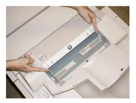
3. Load the paper/tabs, aligning it to the front side of the tray.
