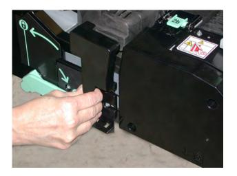
5. Grab and lift the amber-gold colored handle only, lift, and pull up and out of the transfer module.
