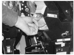
4. If necessary, the staple cartridge unit as shown and remove the jammed staple.
