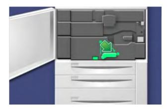
3. Carefully pull out the transfer module.
