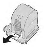
6. While holding the tabs of a new staple cartridge, push it into the unit.
