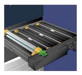
8. Remove the old charge corotron by holding the amber-gold colored casings provided at the both ends of the charge corotron and gently pulling straight up.
