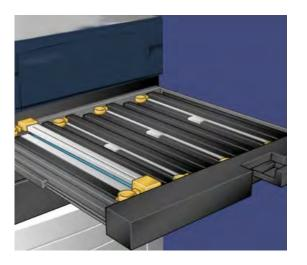
7. Grasp both of the amber-gold colored casings on the old charge corotron and push towards the back of the machine. A clicking noise indicates that it is being released.
