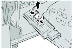
5. Remove the jammed staples from the cartridge.
