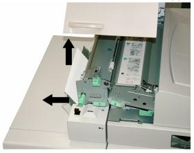
3. Move handle 1a to the left, rotate the knob 1c, and remove any jammed paper.
