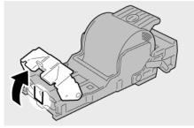
5. Move the lever on the rear of the staple cartridge unit in the downward direction.
