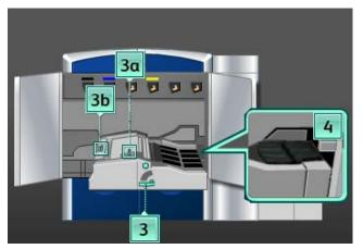
1. Open the left and right front doors (print engine left side).
