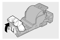
6. Reinstall the cartridge unit to its original position in the finisher.
