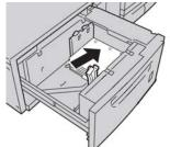
**6.** Adjust the paper guides by pressing in the guide release and carefully moving the Edge Guide until it lightly touches the edge of the material in the tray.
