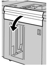
**3.** Lift the green handle(s) and/or rotate the green knob and remove all paper in the entrance area.
