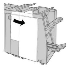
**3.** Pull out the folder output tray (**2d**), swing lever the **2g**, and remove the jammed paper.
