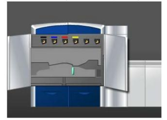
**2.** Use a damp, water-moistened (not wet), lint-free cloth to clean the paper path only in the green lever jam clearance areas as shown in the illustration.
