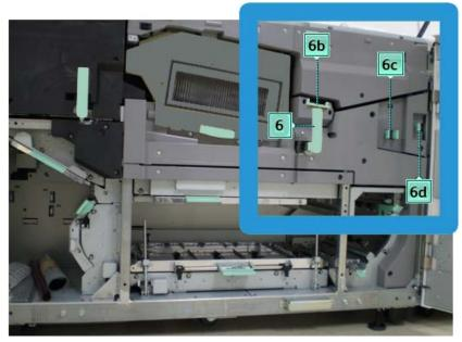
1. Open the left and right front doors (print engine right side).
