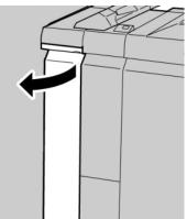
3. Move lever 1a downward and turn knob 1c left. Remove the jammed paper.
