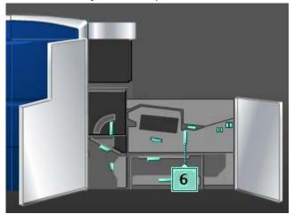
**3.** Use a damp, water-moistened (not wet), lint-free cloth to clean the paper path only in the green lever jam clearance areas as shown in the illustration.
