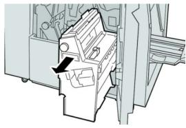
**4.** Turn the knob **4a** to remove the jammed paper from the left side of unit **4**.
