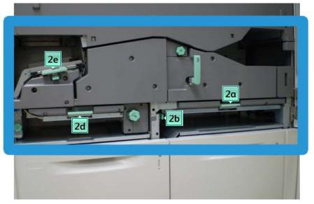
1. Open the left and right front doors (print engine left side).
