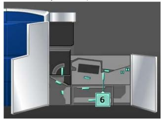
3. Lift levers **6a** and **6b** and remove the jammed paper.
