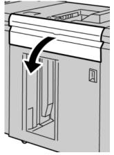
2. Lift the green handle and/or rotate the green knob and remove all paper in the entrance area.
