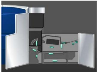
2. Lift lever **7g** and move it to right to remove jammed paper.
