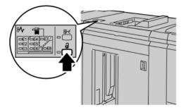
Wait until the Unload indicator lights and then open the HCS front door.
