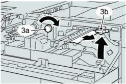
**3.** Lift the green handle and/or rotate the green knob and remove all paper in the entrance area.
