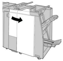
3. Move the levers 3b and 3d; remove the jammed paper.
