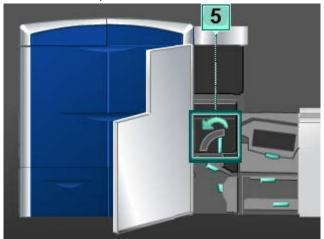
3. Carefully remove any jammed paper on the left side of the fuser.
