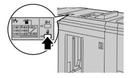
Wait until the Unload indicator lights and then open the HCS front door.
