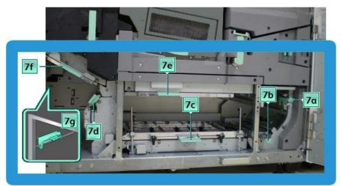
**1.** Open the left and right front doors (print engine right side).
