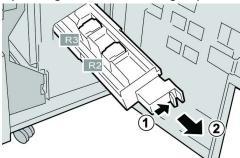
**4.** Hold the tabs of the staple cartridge unit by the tabs and lift to remove it.
