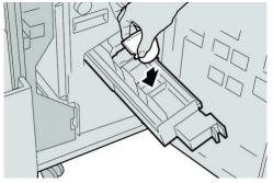
6. Push the staple cartridge unit to its original position in the machine.
