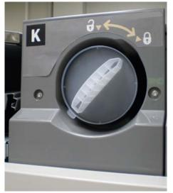
4. Remove and dispose of the empty cartridge according to local regulations.
